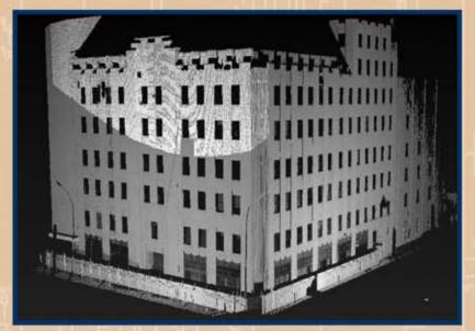
Scans were taken at ground level with our long range scanner, providing a digital map of the façade. High resolution scans were done on a portion of the upper façade areas, to increase data complied.
