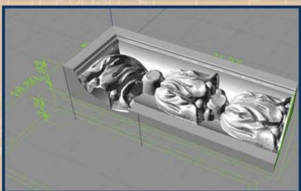
Digital restoration of the scan of the architectural element – restored to its original condition.
